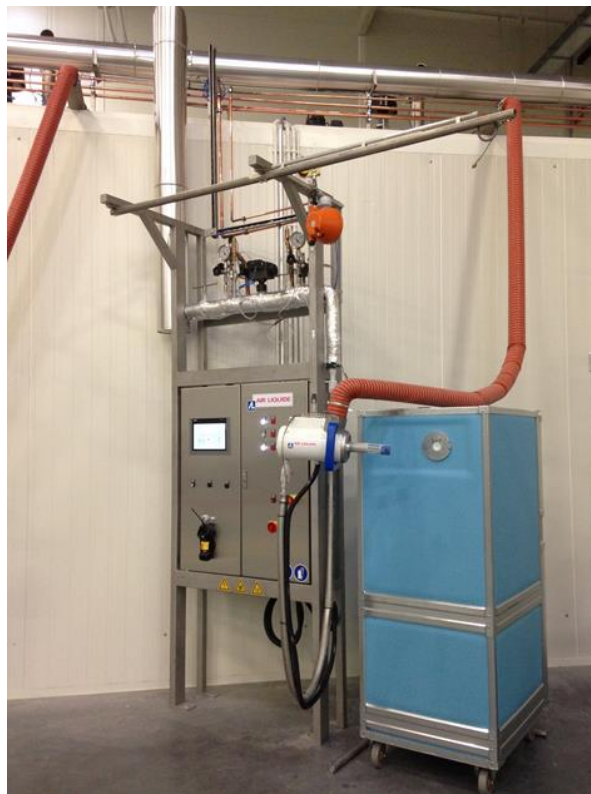
Using the Carbofresh filling system, the cooling agent reaches the slide-in cooling module within a few seconds.
