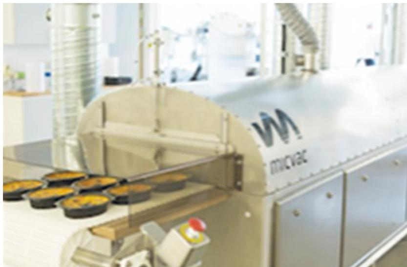
The Micvac pilot plant in Gothenburg, Sweden. Customers can test the process, develop recipes and produce small test quantities.
