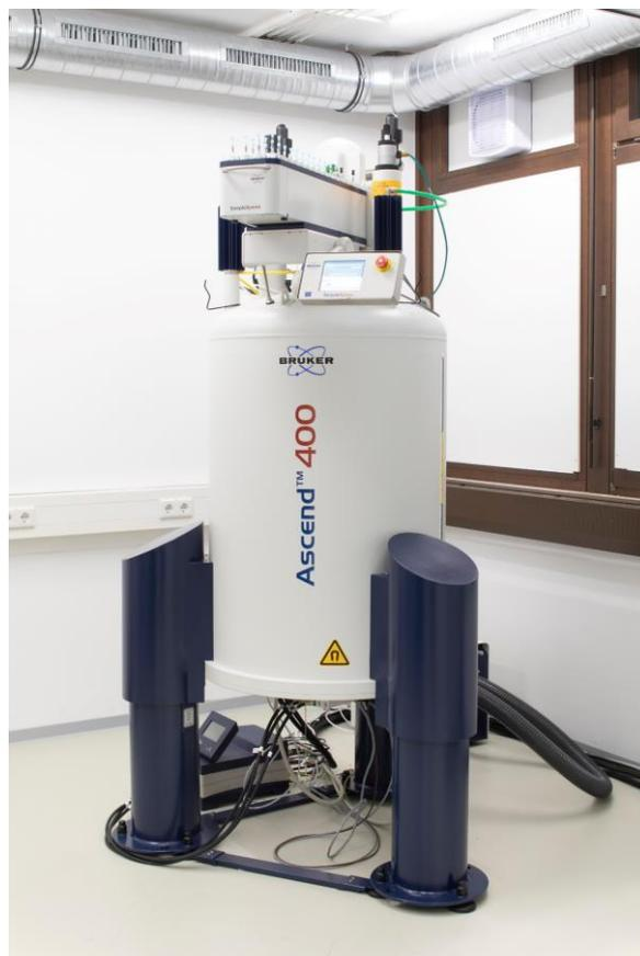
The new NMR spectrometer at the DIL is already being used in ongoing research projects. Within the cooperative project “BioanBak”, antibacterial compounds from pine heartwood were identified via NMR spectroscopy and a quick test was developed to assure the quality of antibacterial pine heartwood.
