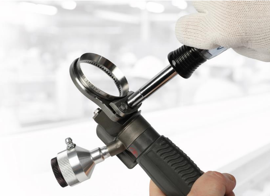
Quantum Flex unique quick-change blade house with cam mechanism.
