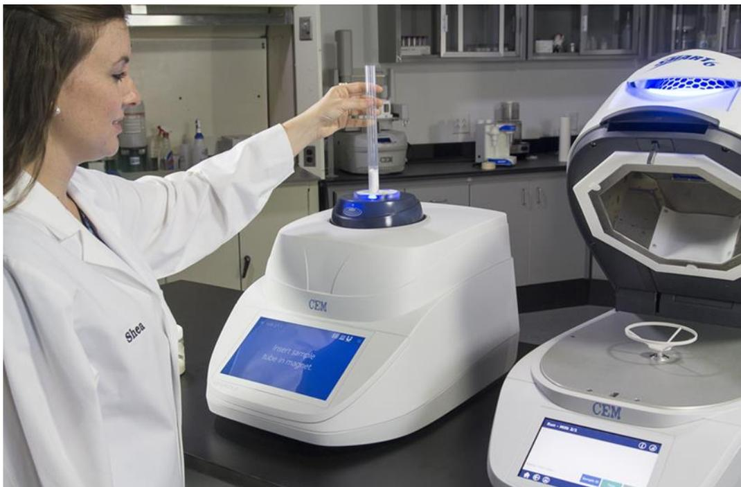
Fig. 2: Transfer of the dried sample to the NMR nuclear resonance spectrometer (Trac-Module)
